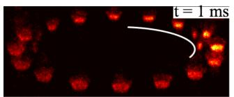
Figure 1: Azimuthal thermo-acoustics instabilities in the MICCA annular combustor [1-5]
