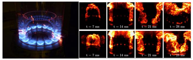
Figure 1: MICCA laboratory scale annular combustor (CNRS/EM2C) [1-6]
